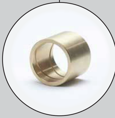
TYPE 2: SAE660 GREASEABLE BRONZE WITH FIGURE 8 GREASE GROOVE
